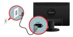
Connect the power cord for your monitor to the power port on the back of the monitor.
